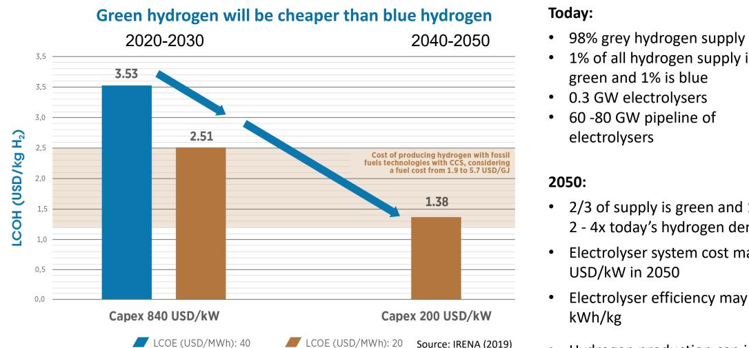
**Key assumptions electrolyser:** Load factor: 4200 hours (48%), conversion efficiency 65% (today), 75% (2050)
